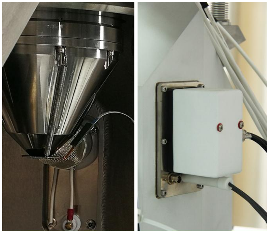
SE: High Vacuum Secondary Electron Detector (With Detector Protection)
