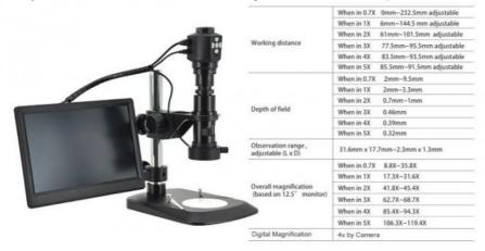
4. A36.4952 is equipped with the external coaxial light, which can uniformly illuminate the surface of the plane and the shiny surface, and enhance the features of marking, recessing or embossing. It can highlight the uneven surface of the object, overcome the interference caused by the reflection of the surface, and improve the microscope reproducibility.
