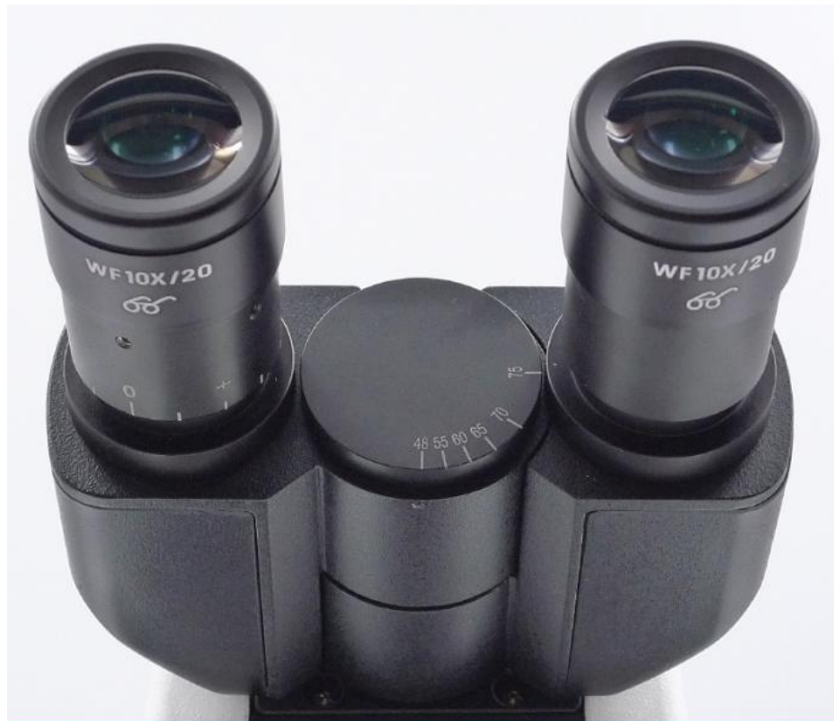
Seidentopf Head Inclined 30° Rotatable 360° , Interpupillary Distance 48-75mm
