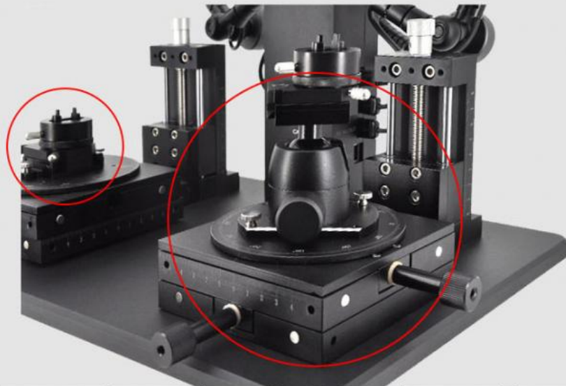
○ High Precision Double Layer Square & Round Working Stage Manual Control X/Y/Z/R Free Movement
