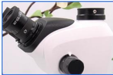
A53.2650-E50P50 Trinocular Head Inclined 35° , Light Split Fixed E50:P50 (Optional)
