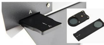
With Micrometer X-0.1mm*180 Div / Y-Single Line
