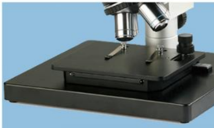
Metal Base 300*250mm, Mechanical Stage 160*140mm, Moving Range 35*30mm, X/Y Coaxial Moving Knob On Stage For Convenient Operation
