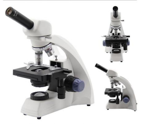
▲ A11.1531-M Monocular Head Biological Microscope
