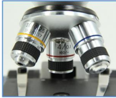
Backward triple revolving nosepiece Achromatic 4x,10x,40x
