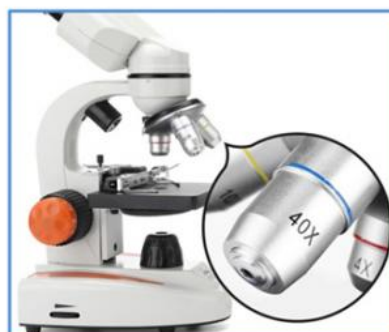
Backward triple revolving nosepiece, Achromatic 4x,10x,40x
