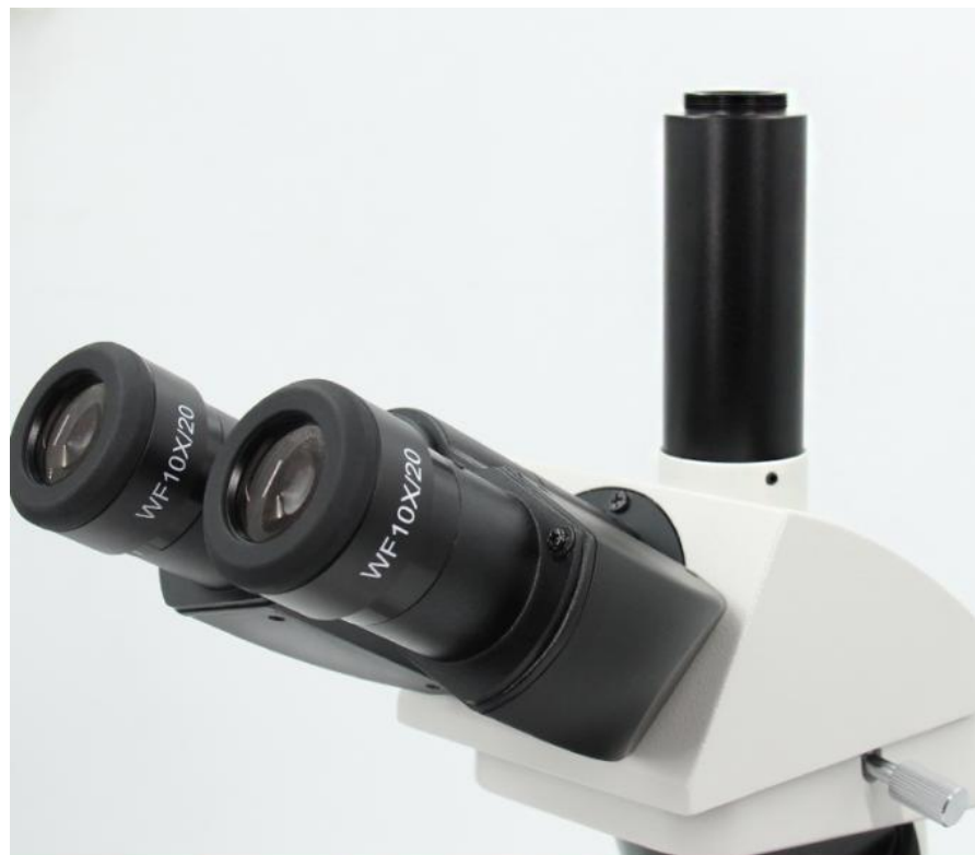
Seidentopf Trinocular Head, 30° Inclined, 360° Rotatable, Interpupillary 48~75mm, Wide Field WF10x/20mm, Dia.30mm
