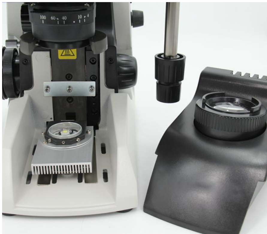
Halogen Lamp 12V/20W, Brightness Adjustable Light Source Cover Removable For Easy Repair
