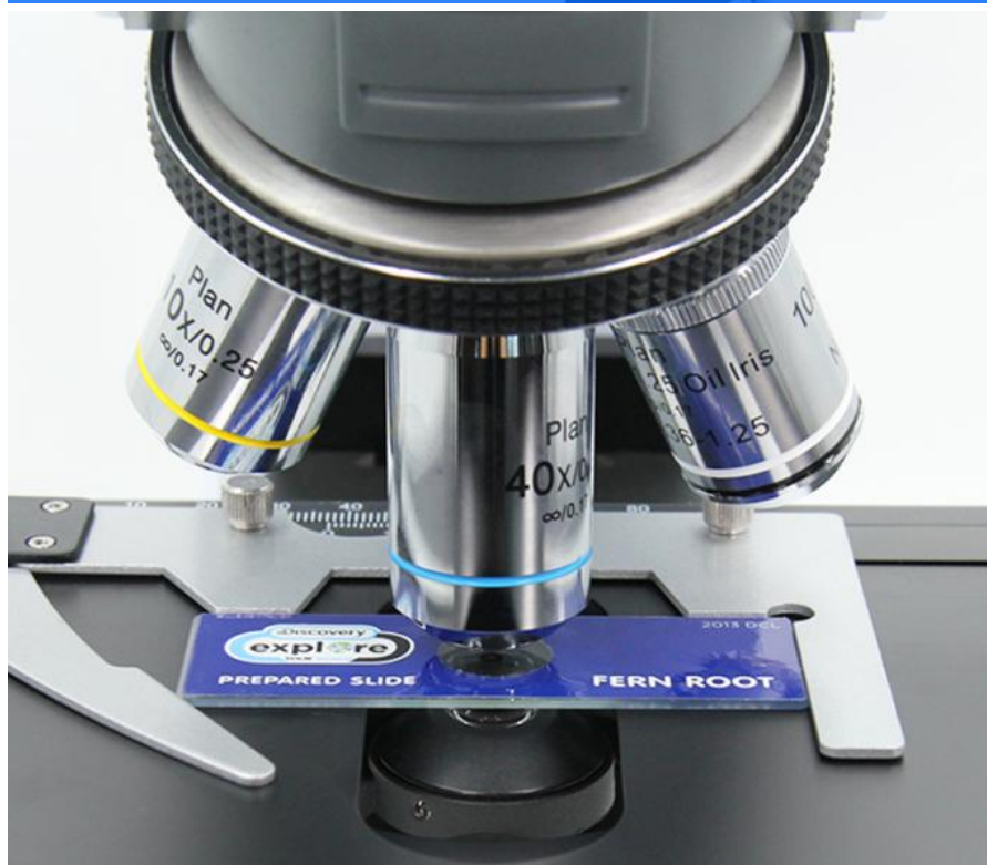
Backward Quintuple Nosepiece, With Slide Slot Infinity Plan Achromatic Objective 4x,10x,40x,100x
