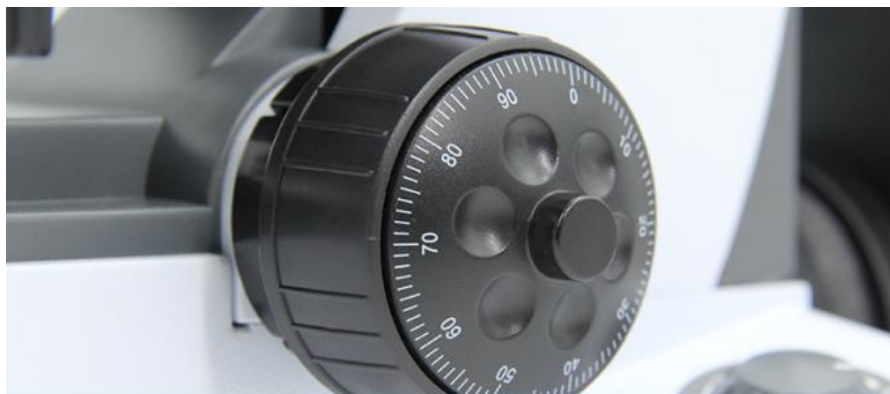
Coaxial Coarse & Fine Adjustment, Focusing Range 24mm, Fine Division 0.001mm, Coarse Stroke 37.7mm, With Lock
