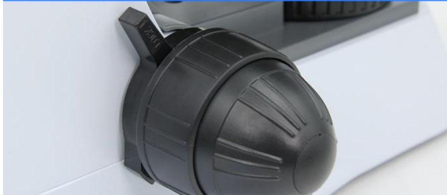
Coaxial Coarse & Fine Adjustment, Focusing Range 24mm, Fine Division 0.001mm, Coarse Stroke 37.7mm, With Lock
