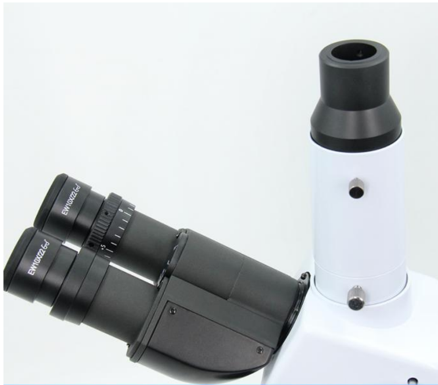
Seidentopf Trinocular Head, 30° Inclined, 360° Rotatable, Interpupillary 48~75mm, Left Eyepiece Tube Diopter Adjustable
