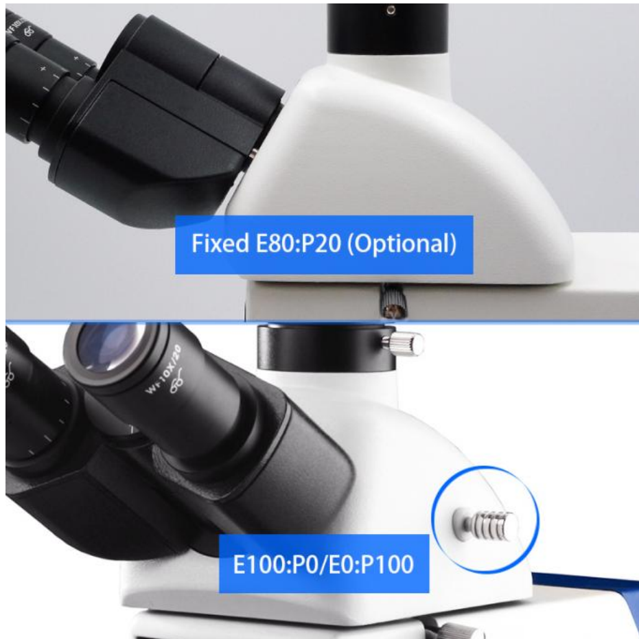
Trinocular Head Light Split Optional Between Switch E100:P0/E0:P100 And Fixed E80:P20 In Fixed Light Split, Eyepiece 80% : Photo 20% User Can View Image At Same Time In Both Path In Switch Light Split, Eyepiece 100%:Photo 0% / Eyepiece 0%:Photo 100%, Camera Can Have 100% Light For Photo Capture.
