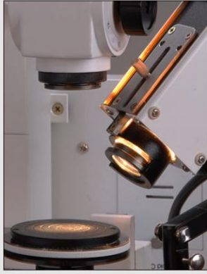
○ Polarizing Light Lens Set, To Eliminate Flare Lights And Dazzling Lights.
