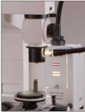
○ Coaxial Light Attachment To Get Vertical Light Path For Watching Inside Deep Hole Bottom
