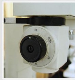
Magnification Switch, For 5 Step Zoom Plan Objective 0.8X, 1.2X, 2X, 3.2X, 5X
