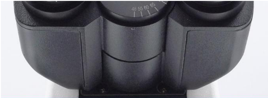
Seidentopf Head Inclined 30° Rotatable 360° , Interpupillary Distance 48-75mm
