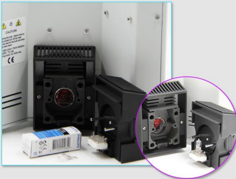
○ Light Source Cover Can Be Removed Easily To Change Bulb
