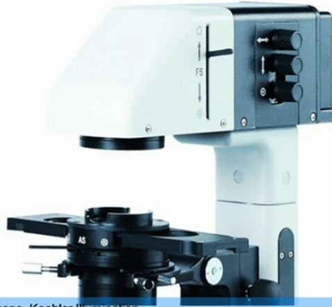
A14.0900 Inverted Microscope, Koehler Illumination Built-in Kohler illuminator, The Condenser Bracket Can Be Rotated 30 Degree, Swivel Bracket With The Orientation and Locking Device, With Iris Diaphragm and The Center of Filament Can be Adjusted N.A.0.3 Working Distance 72mm, for 4x- 40x Objectives N.A.0.5 Working Distance 28mm, for Higher Magnification Objectives
