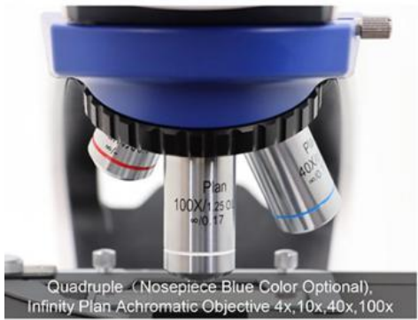
Trinocular, 45 ° tilt, Adjustable Pupillary Distance 52mm-76mm, 0.4x C-Mount, PL10X22mm
