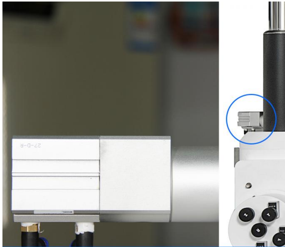
The Isolating Valve Ensures That The Upper Vacuum Is Not Affected When The Sample Room Is Opened
