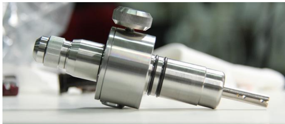
3 Molybdenum Objective Apertures, Adjustable Outside Of Vacuum System, No Need Disassemble Objective To Change Aperture
