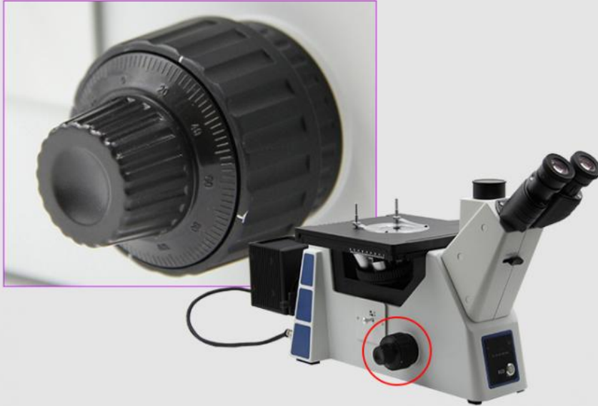
○ Coaxial Coarse & Fine Focusing System With Adjustable Tension, Coarse Range 9mm (6.5mm up & 2.5mm down), Fine Precision 2 \mu m
